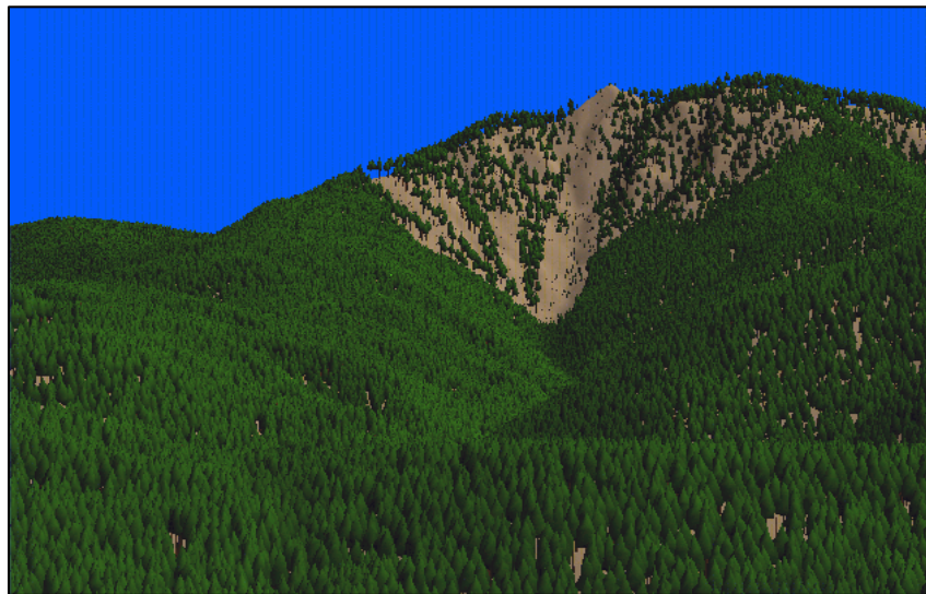
Figure 1. This sample 3-D visualization utilizes geometric modeling techniques to render trees on the surface. Trees have been rendered using a standard cone symbol for coniferous trees, but placement and sizing of the objects respects polygon source inventory characteristics. Shadowing is included for each tree object providing a more realistic look. Image courtesy of Robert J. McGaughey, USFS, Pacific Northwest Research Station.
