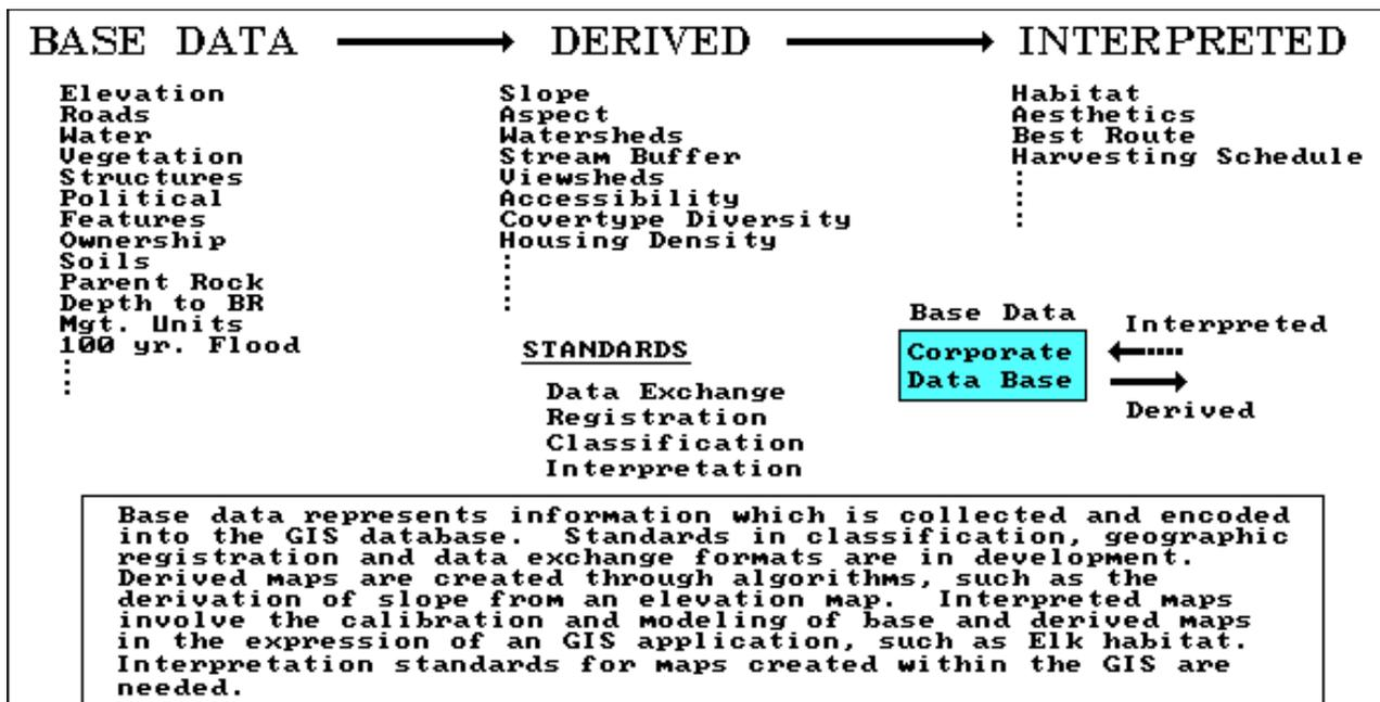
This figure describes the basic data types that are used and created by a GIS.
