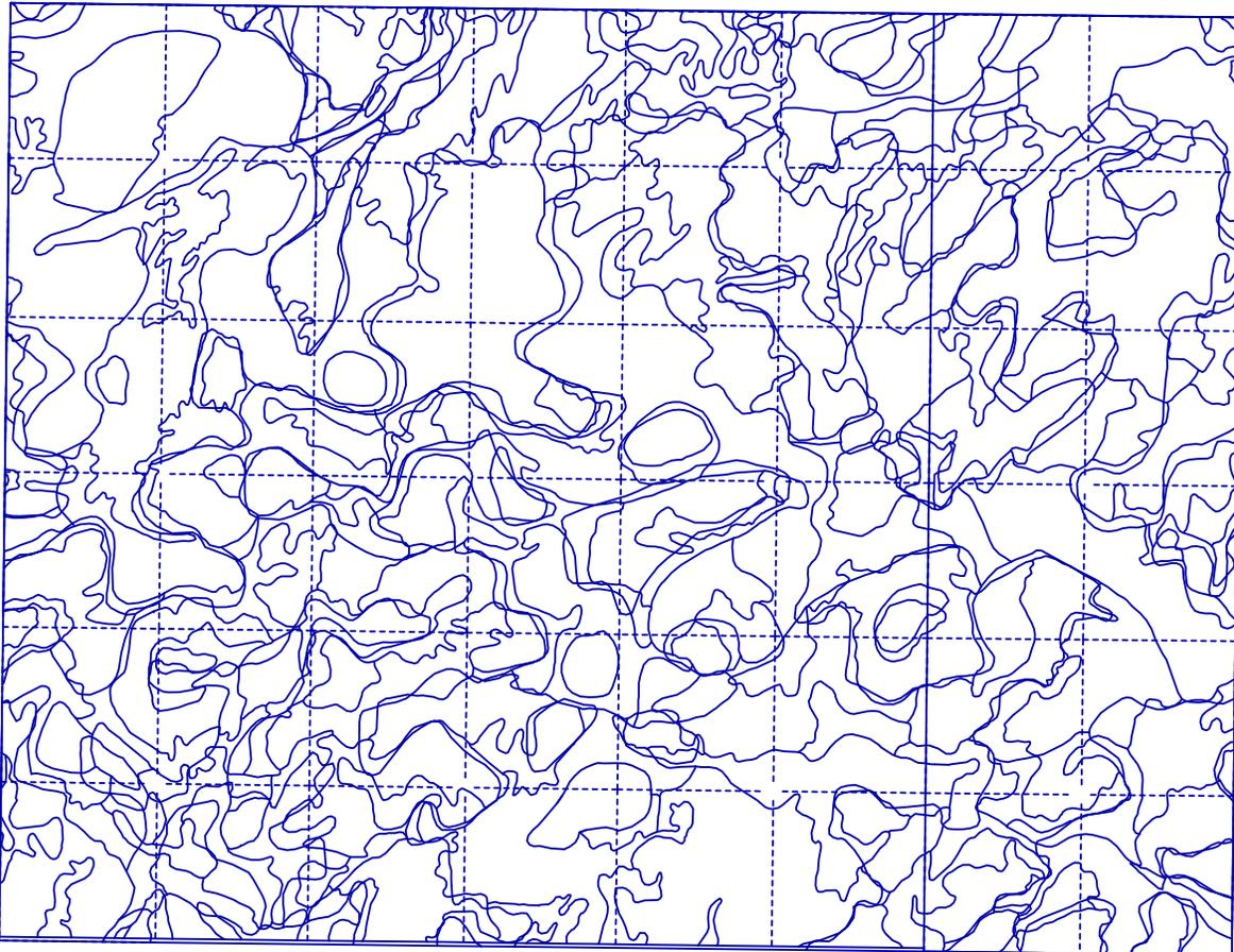
**Example 1: Map 8 - The new polygon data layer constructed by overlaying the SOIL layer with the FOREST layer. This layer contains 901 polygons. Note the existence of numerous sliver polygons indicating an accuracy and/or scale mismatch between the original data sets.**
