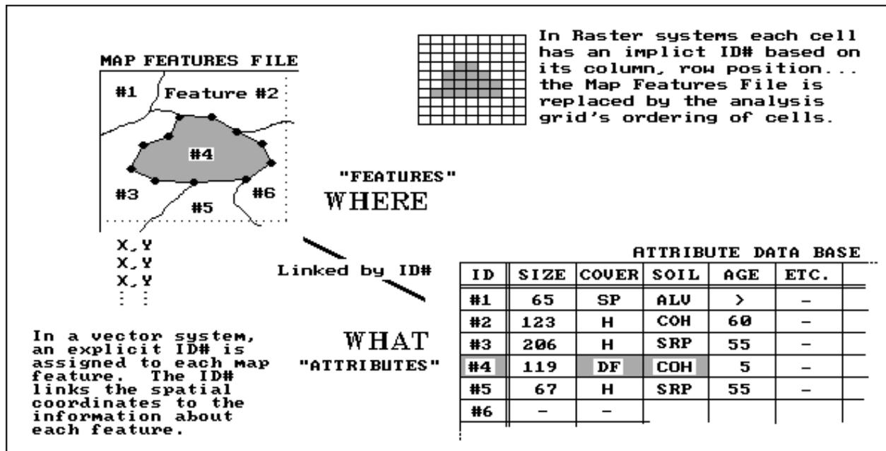
This figure illustrates the basic linkage between a vector spatial data (topologic model) and attributes maintained in a relational database file.
