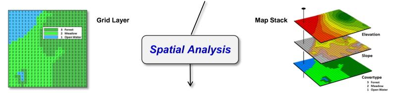
**Spatial Analysis** extends the basic set of discrete map features (points, lines and polygons) to map **surfaces** that represent continuous geographic space as a set of contiguous grid cells (matrix), thereby providing a **Mathematical Framework** for *map analysis* and *modeling* of the
