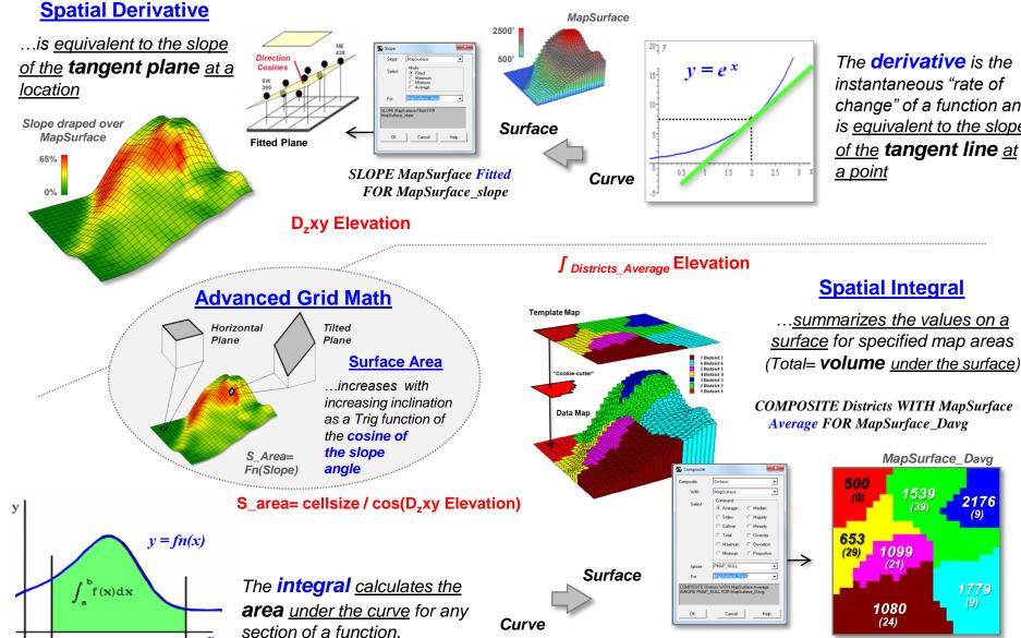
The **derivative** is the instantaneous "rate of change" of a function and is equivalent to the slope of the **tangent line** at
