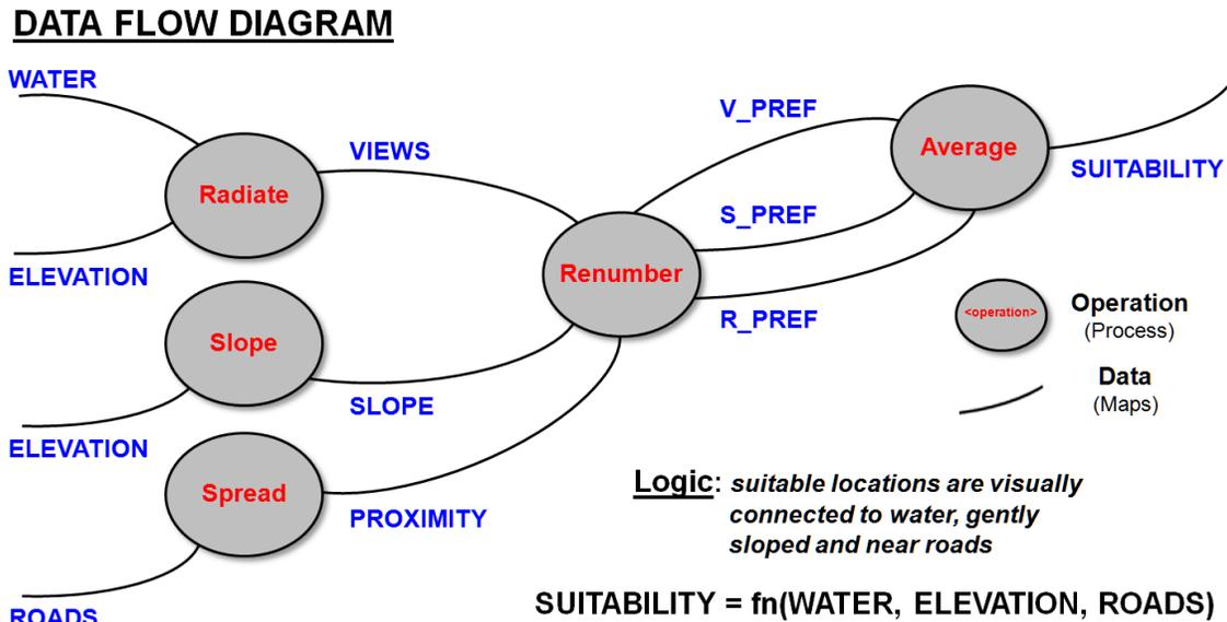
*Figure 1. Example of a Data Flow Diagram emphasizing the processing steps used in converting one data set into another (Lines= processing; Ovals= maps).*
