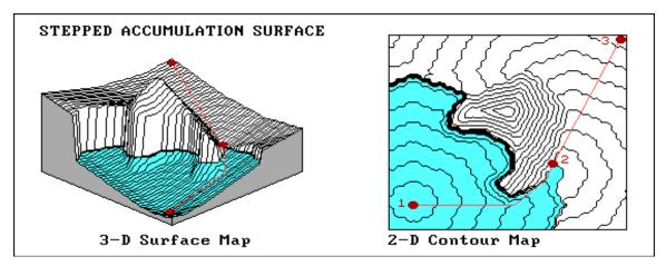
Figure 25.4. Stepped Accumulation Surface. Proximity from the first point is calculated (shaded) until the second point is reached, then proximity from that point is calculated (non-shaded) forming the next tier; the individual optimal paths along each of the stepped proximity surfaces forms the overall optimal route.
