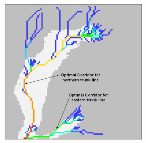
Figure 3. The optimal corridors for routes serving numerous end points indicate the spatial sensitivity in siting trunk lines.
