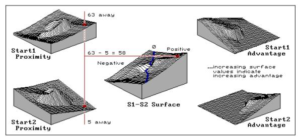
Figure 1. The difference between two proximity surfaces identifies the relative geographic advantage between two locations.
