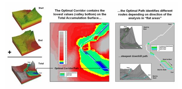
Figure 1. "Flat areas" on the valley bottom of the Total Accumulation Surface (blue) are the result of artificial differences in optimal paths induced by grid-based distance measurement restriction to orthogonal and diagonal movements.
