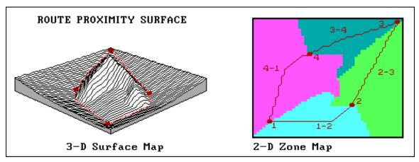
Figure 2. Route Proximity Surface. Proximity from the optimal route identifies the distance to the closest segment of the route for every location in a project area; the influence zone of each segment along the route identifies which segment is the closest.
