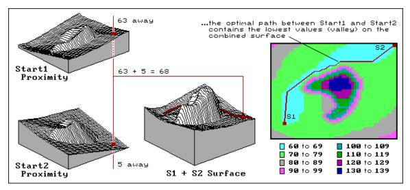
Figure 1. The sum of two proximity surfaces identifies the optimal path between two locations as the lowest values, while increasing values identify the "opportunity cost" of forcing a path through any location.
