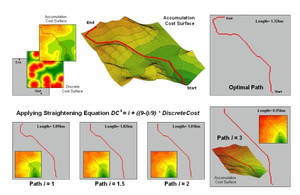
Figure 2. Examples of Applying the LCP Straightening Equation.
