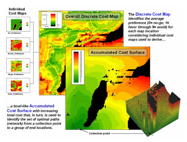
Figure 1. Relative preferences are used to identify the minimal overall cost of constructing a route from a collection point to all accessible locations in a project area.
