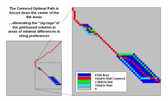
Figure 3. Comparison of directional optimal paths and the centered optimal path.
