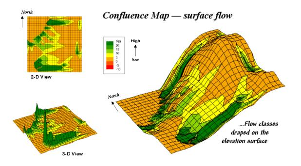
Figure 2. 2-D, 3-D and draped displays of surface flow confluence.
