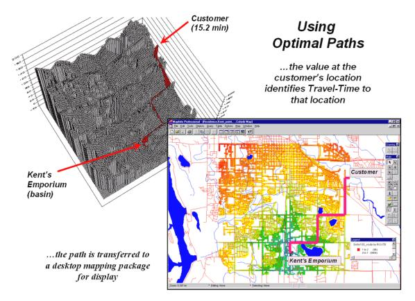
*Figure 2. The optimal path (quickest route) between the store and any customer location can be calculated then transferred to a standard desktop mapping system.*
