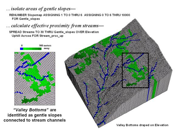
Figure 3. Valley bottoms are identified as flat areas connected to streams.
