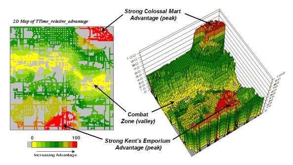
*Figure 3.* A transformed display of the difference map shows travel-time advantage as peaks (red) and locations with minimal advantage as an intervening valley (yellow).
