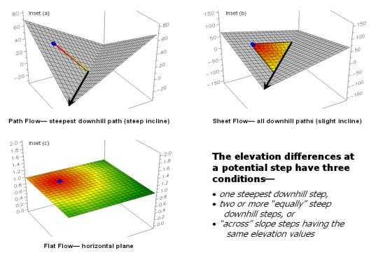
*Figure 2. Surface inclination and liquid type determine the type of surface flow—path, sheet or flat.*
