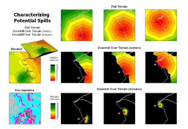
Figure 2. Overland flow can be characterized as both distance traveled and elapsed time.
