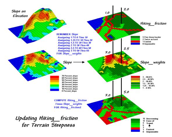
Figure 1. Hiking friction based on Cover Type and Roads is updated by terrain slope with steeper locations increasing hiking friction.
