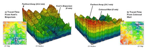
*Figure 1. Travel-time surfaces show increasing distance from a store considering the relative speed along different road types.*
