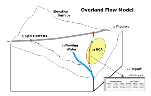
1) The *Pipeline* is positioned on the *Elevation* surface
