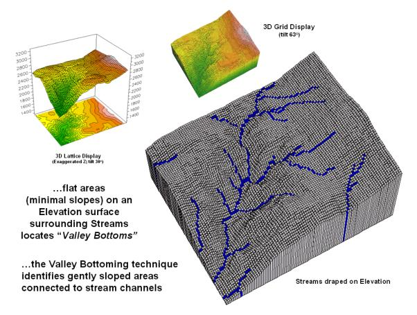
Figure 1. Gentle slopes surrounding streams are visually apparent on a 3D plot of elevation.
