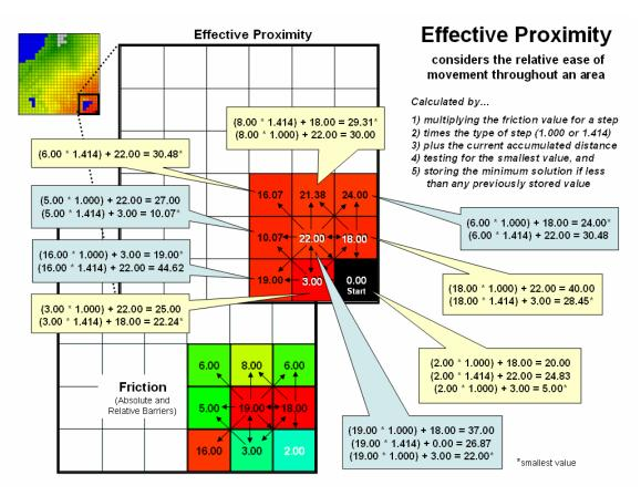
*Figure 2. Effective distance rings advance by summing the friction factors times the type of grid space movements and retaining the minimal accumulated distance of the possible paths.*
