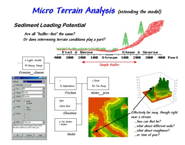
Figure 2. Extended erosion model considering sediment loading potential considering intervening terrain conditions.
