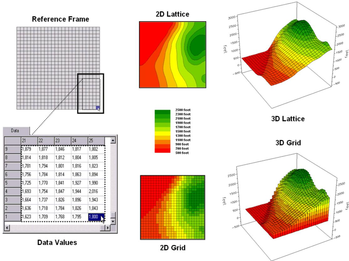
Figure 1. Grid-based data can be displayed in 2D/3D lattice or grid forms.
