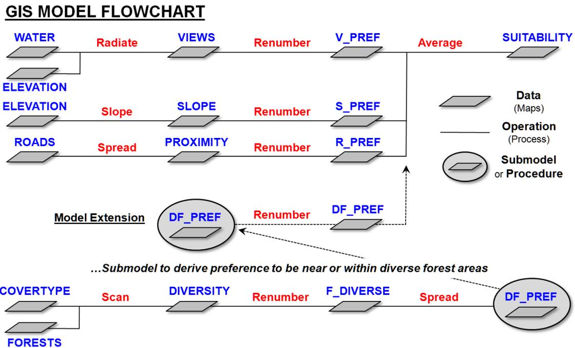
Figure 2. Example of a GIS Model Flowchart where maps (i.e., data sets) are depicted as "floating boxes" and operations (i.e., processing steps) are depicted as lines.
